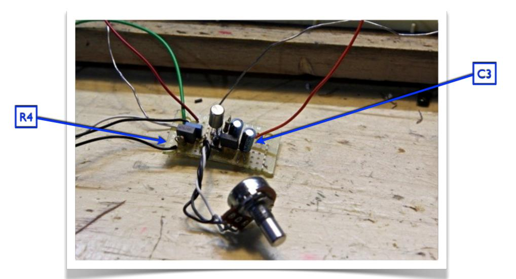
Connect the IM resistor (R4) between the cluster of wires at the input and ground. Place the other 22u electrolytic cap (C3) between the positive and negative busses. Place the IN4001 diode (which I cleverly forgot to include in this photo) alongside it, with the banded end connected to the positive bus.
