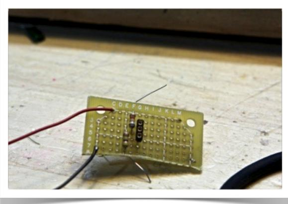
Here I've used a piece of SIP socket to house the transistor. The advantage: You can audition different transistors after the circuit is built, and you don't have to solder the relatively fragile and valuable germanium transistor. It's a major pain unsoldering anything from perfboard if you install it incorrectly!
