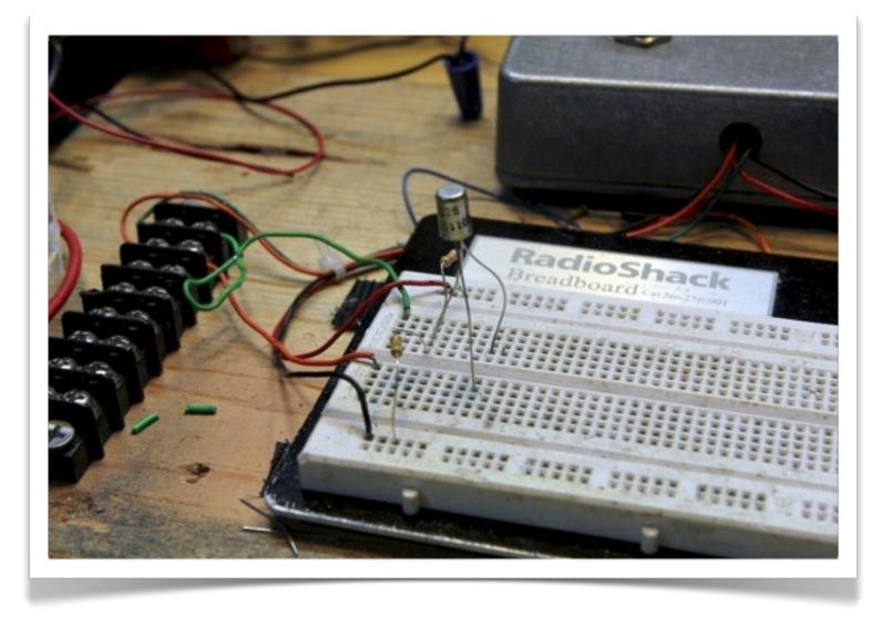
Connect the transistor's base to the power bus using a 68K resistor. Connect the base to ground using a 470K resistor. (In other words, you'll have three wires on the same bus.)
