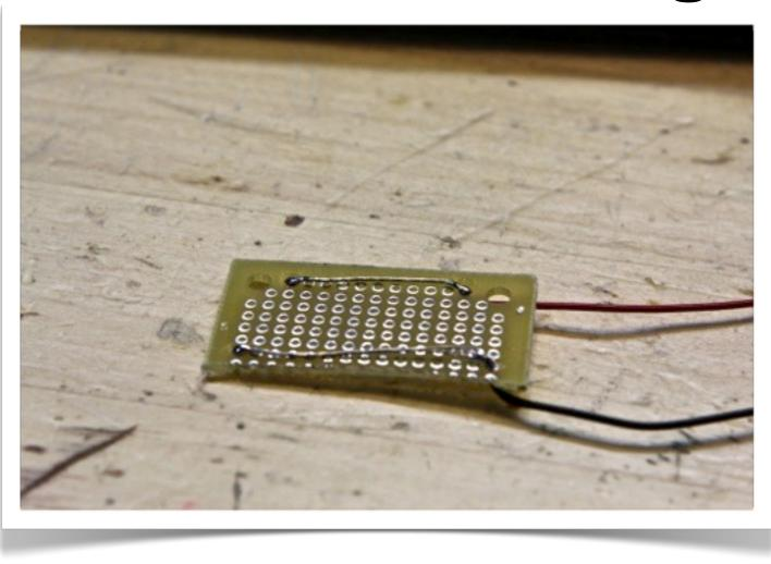
Prepare a piece of perfboard about this size. Strip several inches from a pair of wires and solder them loosely in place for your positive and negative busses.
