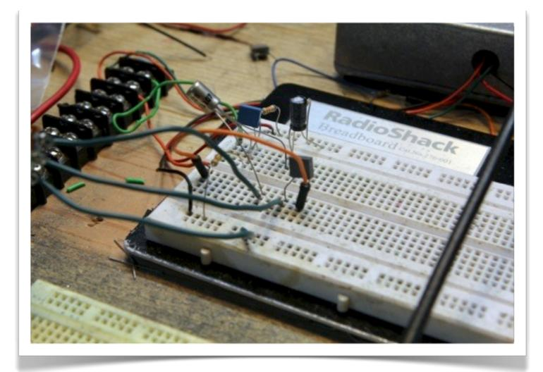
Replace the 472 input cap with the larger 104. The effect should become a much more loud, deep, and distorted. (Don't be fooled by the physical cap size — the small blue cap in the pic above is actually of larger value than the fat gray one in the previous pics.)
