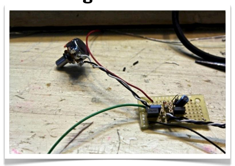
Whether you use two tone pot wires or three, connect lugs 3 and 2 to the leftmost leg of the 104 cap (C4). Attach an input wire to the same location. Connect the lug I wire to the leftmost leg of the 473 cap (C1).
