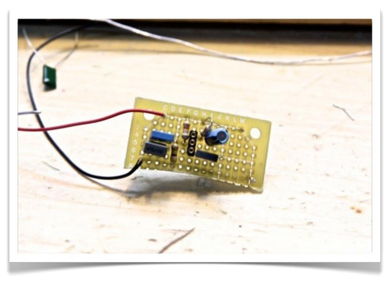
Connect one leg each of R3 and and C3 to the positive bus, and the other legs to the topmost transistor socket pin.
