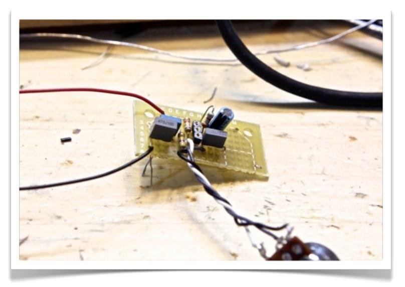
Connect the wire from the A50K pot's lug 3 to the bottom pin of the transistor socket. Connect the wire from lug 1 to ground. Connect the wire from lug 2 to the leftmost leg of C3.
