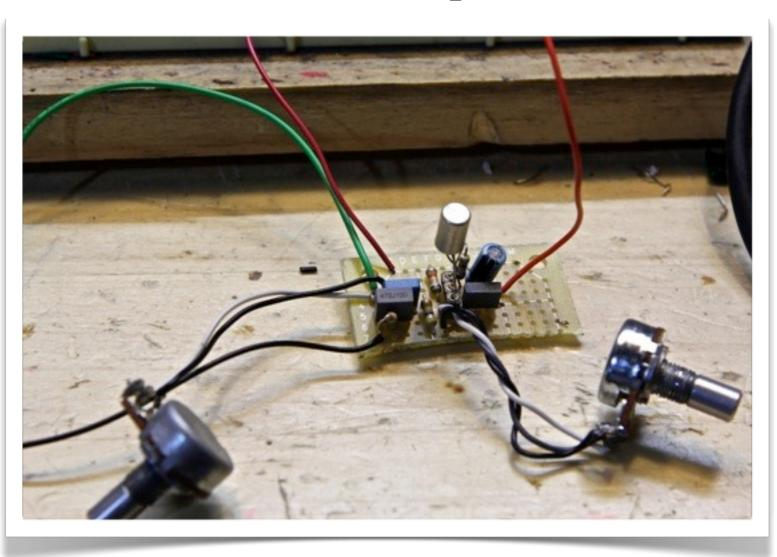
Connect an output wire to the rightmost leg of C2.
