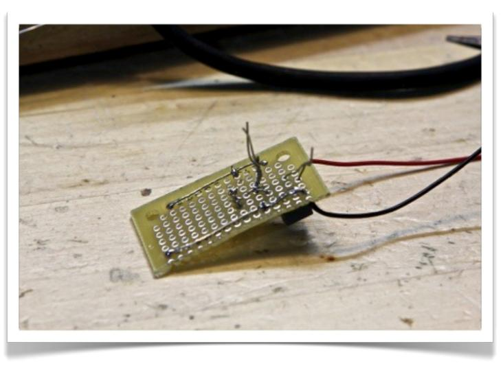
The reverse side of the perfboard will inevitably look like a bloody mess. Just be careful not to let wires touch where they shouldn't. It takes some soldering finesse to connect all those wires to the middle pin of the transistor socket without letting the solder spill over onto the other two socket pins. (This is the part of the project where you'll most regret socketing instead of just soldering in the transistor.)
