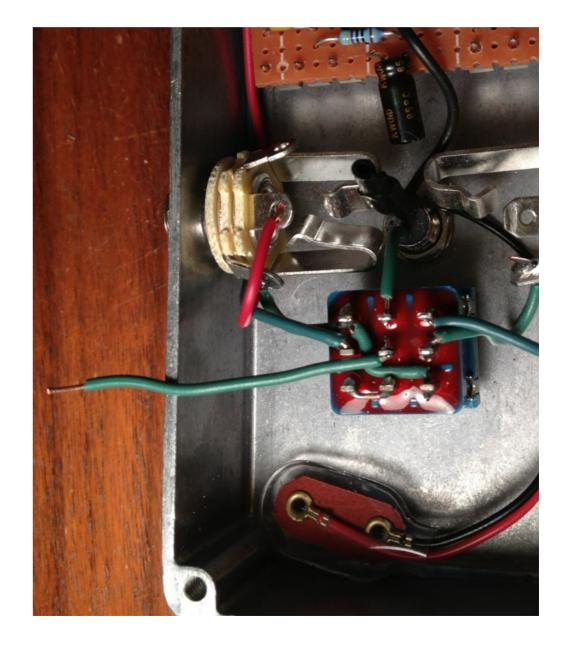
Solder the other end of this wire to the input jack's innermost lug **together with** the circuit board's +9v wire (the one connected to the hole at row A/ column A).
