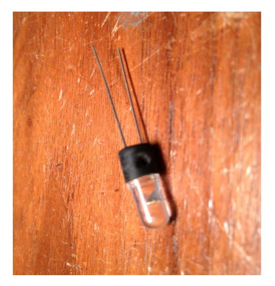
Press the LED and stopper into the LED bezel, securing them in place.
