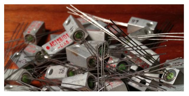
the description use AC128 germanium types. For a silicon Fuzz Face sound, 2n3904 transistors work well and are easy to find.
